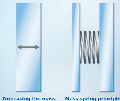
Higher sound insulation factors can be achieved by increasing the thickness of the glazing and ensuring it is asymmetrical. The frequency response curves of two panes combined to form a mass-spring system in insulating glass add up to better sound insulation.
