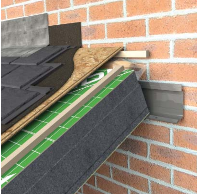
Gable extended soffit overhanging side frames
