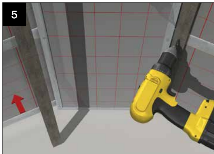
Attach timber battens at every strut position using dry wall screws. BATTENS SUPPLIED IN PACKS, NEED TO BE CUT ON SITE TO SUIT.
