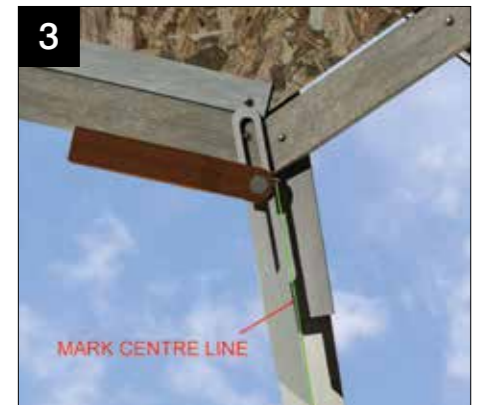
Use an angle finder to determine angle of each hip bar.
