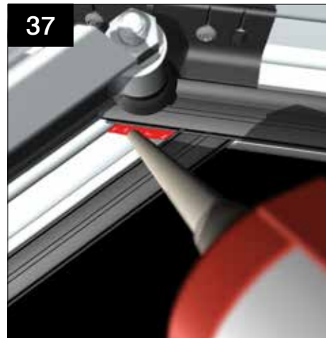
Seal the area where the co-extruded gasket on the hip bar butts against the co-extruded gasket on the jack rafter.
