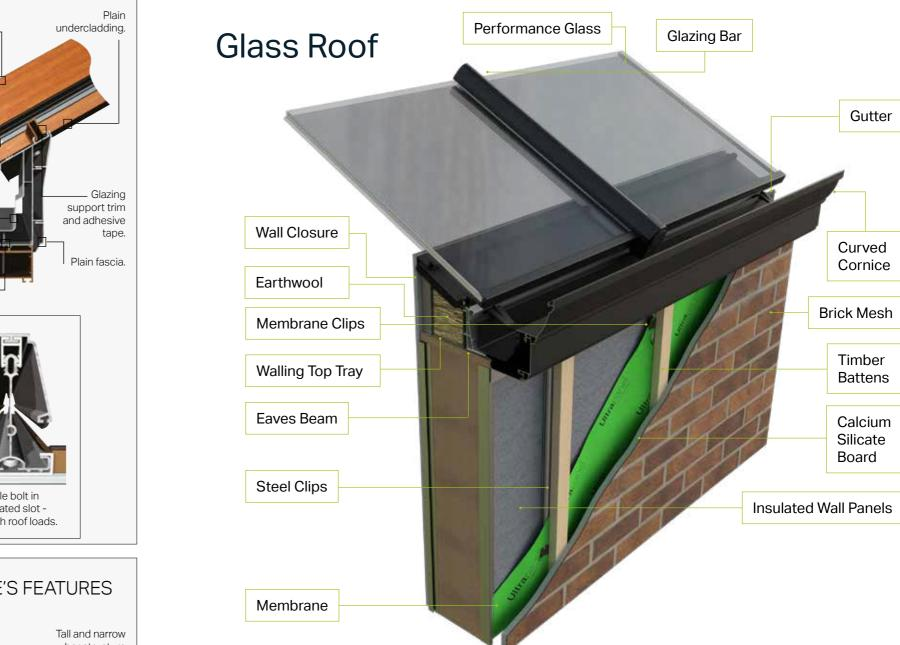
The Glass Roof is available with the hup! walling system from Ultraframe. The Glass Roof can be supplied with a hup! mini pelmet as shown below, or the internal pelmet can be widened to up to 1200mm making it the perfect place for spotlights or speakers.
